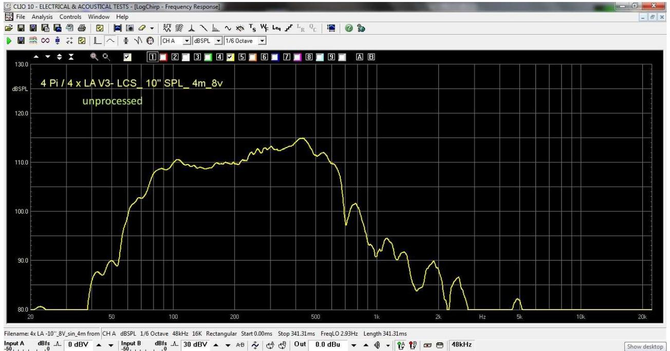
Figure 9a. LO Section - Frequency Response of LO Section of 4xLA V3, free space (4xPi), 8Vrms, at 4m on axis, unprocessed
