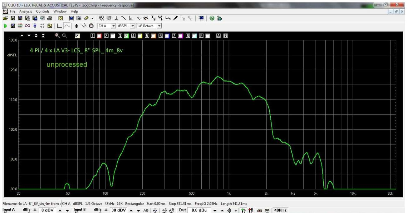
Figure 9b. MID Section - Frequency Response of MID Section of 4xLA V3, free space (4xPi), 8Vrms, at 4m on axis, unprocessed
